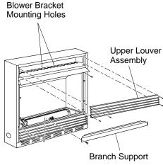
Figure 15 - Removing Upper Louver Assembly and Branch Support
